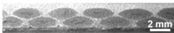
Figure 2 Digital photograph of unidirectional continuous carbon fiber reinforced epoxy, showing groups of carbon fiber and resin bridges between them.
